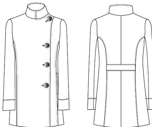
Fig. 3. The transformation of basic patterns in model pattern (Offset buttons model)
