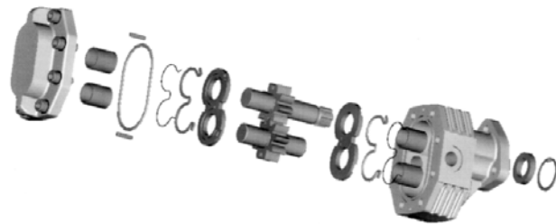
Figure 10: View of gear pump with housing of NL (dismantled with the basic parts)
