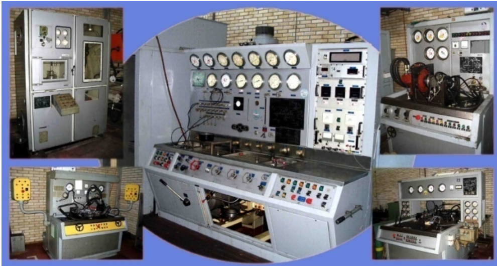
Figure 11: View of universal test stands for testing of hydraulic devices
